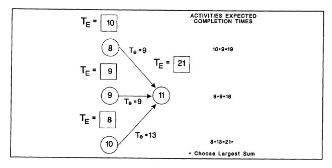
Figure A-7 Calculating  $T_{\rm E}$  with Various Activity Arrows at One Event
