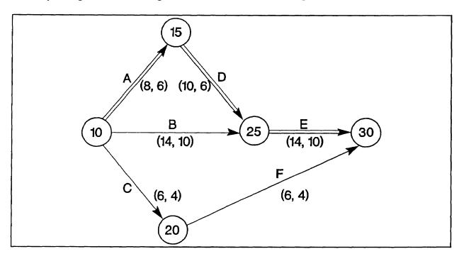
Figure A-12 Normal CPM Network Diagram
